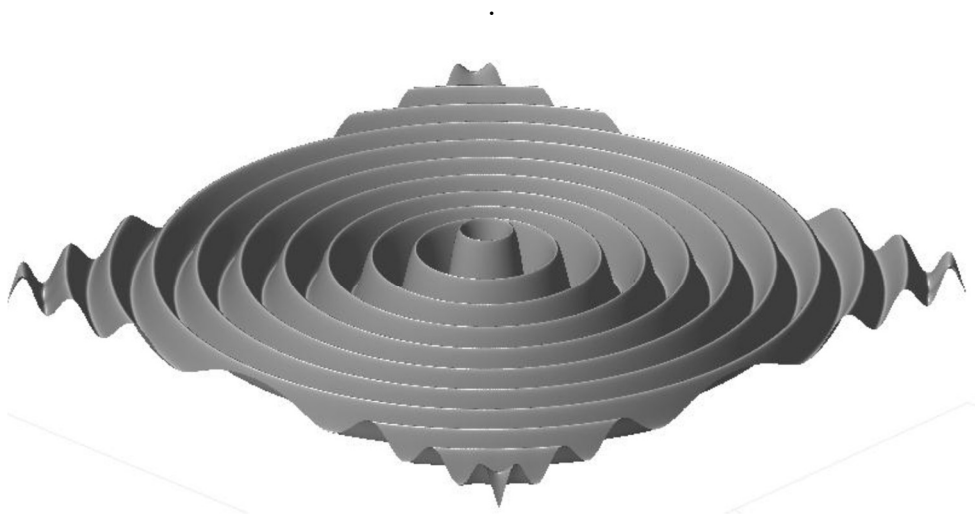
Fig.7 3-D view of the simulated pattern in which \lambda = 442nm , \varphi_i = 2^\circ for 90 rotations
