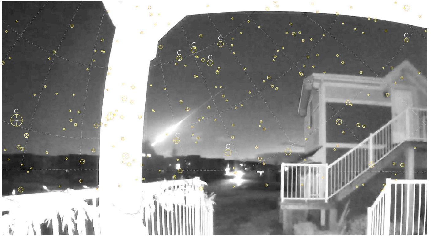
Extended Data Fig. 4 | Cochrane security camera astrometric calibration. Composite of frames from the Cochrane security camera video showing the fireball and the calibration stars (marked with a white letter C), four of which were in Cassiopeia. An equatorial grid is laid over the video with catalogue stars shown as yellow crosshairs. Credit: Airell DesLauriers.
