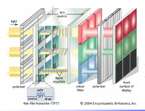
This varying orientation in turn varies the amount of light allowed to pass through the TFT matrix and colour filter, thereby changing the colour picture on the display screen
