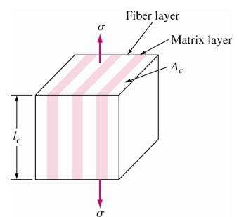
The load on the composite is equal to the sum of the loads on the fiber layers and the matrix layers or  $F_C = F_F + F_M$ . Since  $F = \sigma$  A, we obtain
