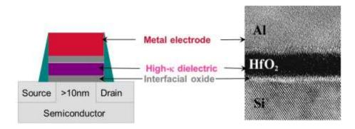
Several different metal electrode materials were introduced instead of previously used heavily-doped silicon. Imagine that you examine several material metal candidates, such as Sc, Ti, Al and Ta, to introduce them into transistor structure. However additional interface layer was also observed at the metal/HfO<sub>2</sub> interface, as indicated by the grey layer between metal electrode and high-k dielectric on the diagram above).
