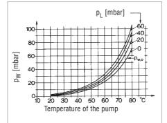
Fig. 2.16 Partial pressure  $p_W$  of water vapor that can be pumped with the gas ballast valve open without condensation in the pump, as a function of the pump temperature for various partial pressures  $p_L$  of air. The lowest curve corresponds to the water vapor tolerance  $p_{W,\,0}$  of the pump
