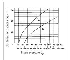
Fig. 2.42 Condensation capacity of the condenser (surface area available to condensation 1 m²) as a function of intake pressure p<sub>D1</sub> of the water vapor. Curve a: Cooling water temperature 12 °C. Curve b: Temperature 25 °C. Consumption in both cases 1 m³/h at 3 bar overpressure
