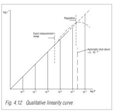
which are to be specified (± 10 % for partial pressure measurement devices).
