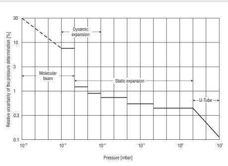
Fig. 3.17 Pressure scale of Federal Physical-Technical Institute (PTB), Berlin, (status as at August 1984) for inert gases, nitrogen and methane
