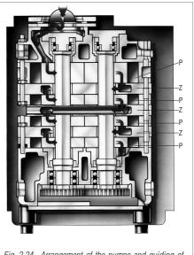
Fig. 2.24 Arrangement of the pumps and guiding of the gas flow. P = Pump stage Z = Intermediate ring
