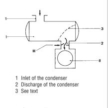
Fig. 2.41 Condenser (I) with downstream gas ballast pump (II) for pumping of large quantities of water vapor in the rough vacuum range (III)
