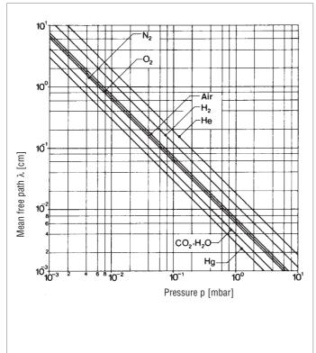
Fig. 9.1: Variation of mean free path  $\lambda$  (cm) with pressure for various gases
