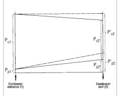
Fig. 2.43 Schematic representation of the pressure distribution in the condenser. The full lines correspond to the conditions in a condenser in which a small pressure drop takes place ( $p_{tot 2} < p_{tot 1}$ ). The dashed lines are those for an ideal condenser ( $p_{tot 2} \approx p_{tot 1}$ ).  $p_D$ : Partial pressure of the water vapor,  $p_L$ : Partial pressure of the air
