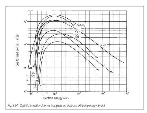
Both the nature of the fragments created and the possibility for multiple ionization will depend on the geometry (differing ion number, depending on the length of the ionization path) and on the energy of the impacting electrons (threshold energy for certain types of ions). Table values are always referenced to a certain ion source with a certain electron energy level. This is why it is difficult to compare the results
