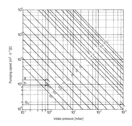
Example: Oil losses for a TRIVAC S 16 A at pressure of 1 mbar:
