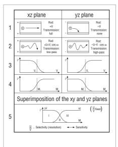
Fig. 4.5 Phenomenological explanation of the separation system
