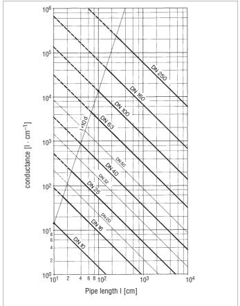
Conductance values for piping of commonly used nominal width with circular cross-section for laminar flow (p = 1 mbar) according to equation 53a. (Thick lines refer to preferred DN) Flow medium: air (d, I in cm!)
