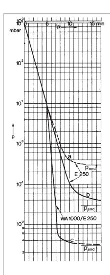
Fig. 2.77 Pumpdown time, t<sub>p</sub>, of a 5 m<sup>3</sup> vessel using a rotary plunger pump E 250 having a nominal pumping speed of 250 m<sup>3</sup>/h with (a) and without (b) gas ballast, as well as Roots/rotary plunger pump combination WA 1001 / E250 for a cut-in pressure of 10 mbar for the WA 1001 (e)
