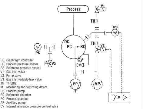
Fig. 3.31 Diaphragm controller with external automatic reference pressure regulation
