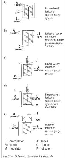
arrangement of various ionization vacuum
