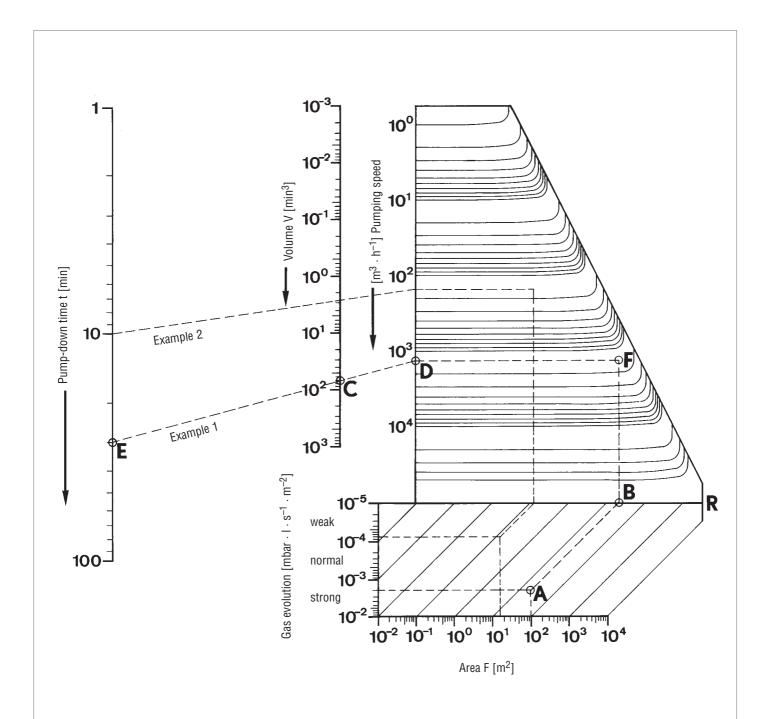
The nomogram indicates the relationship between the nominal pumping speed of the pump, the chamber volume, size and nature of the inner surface as well as the time required to reduce the pressure from 10 mbar to  $10^{-3}$  mbar.
