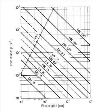
Conductance values for piping of commonly used nominal width with circular cross-section for molecular flow according to equation 53b. (Thick lines refer to preferred DN) Flow medium: air (d, l in cm!)
