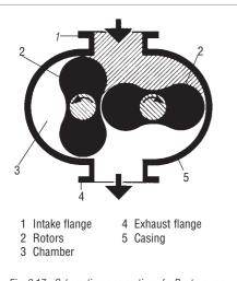
Fig. 2.17 Schematic cross section of a Roots pump
