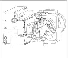
Fig. 2.8b SOGEVAC pump SV 300 with three tangential vanes
