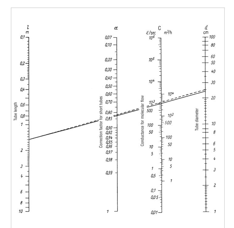
**Example:** What diameter d must a 1.5-m-long pipe have so that it has a conductance of about C = 1000 I / sec in the region of molecular flow? The points I = 1.5 m and C = 1000 I/sec are joined by a straight line which is extended to intersect the scale for the diameter d. The value d = 24 cm is obtained. The input conductance of the tube, which depends on the ratio d / I and must not be neglected in the case of short
