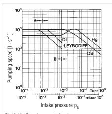
Fig. 2.48 Pumping speed of various vapor pumps as a function of intake pressure related to a nominal pumping speed of 1000 l/s.
