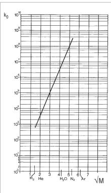
Fig. 2.55 TURBOVAC 450 – Maximum compression  $k_0$  as a function of molar mass M
