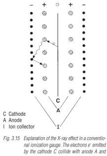
trigger a soft X-ray radiation (photons) there. This radiation strikes, in part, the ion collector and generates photoelectrons e there
