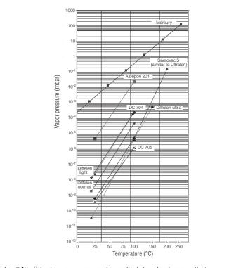
Fig. 9.12: Saturation vapor pressure of pump fluids for oil and mercury fluid entrainment pumps
