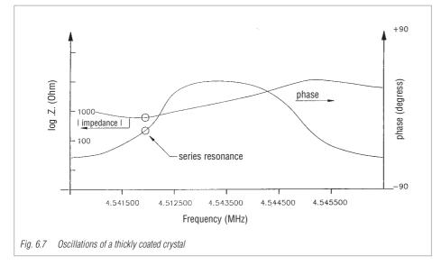
can determine with a phase comparator whether the applied frequency is higher or lower than the crystal resonance point.
