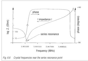
oscillator is created through the sudden phase change that takes place near the series resonance point even with a small change in crystal frequency, see Fig. 6.6.
