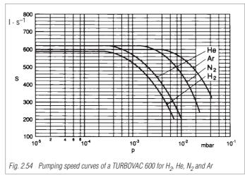
The **pumping speed** (volume flow rate) characteristics of turbomolecular pumps are shown in Fig. 2.53. The pumping speed remains constant over the entire working pressure range. It decreases at intake pressures above 10<sup>-3</sup> mbar, as this threshold value marks the transition from the region of molecular flow to the region of laminar viscous flow of gases. Fig. 2.54 shows also that the pumping speed depends on the type of gas.
