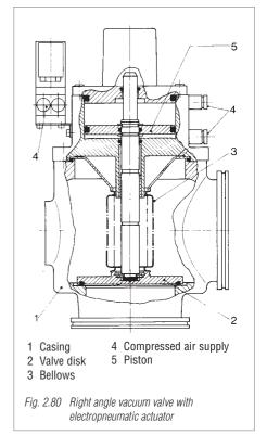
used for highly stringent demands. Their leakage rate is also about 10<sup>-9</sup> mbar · l/s. However, a special case is the pendulumtype gate valve. Despite its grease-covered seal, the leak rate between vacuum and external atmosphere is virtually the same as for bellows-sealed valves because when the valve is in operation the shaft carries out only a rotary motion so that no gas molecules are transferred into the vacuum. Pendulum-type gate valves are not manufactured by LEYBOLD.
