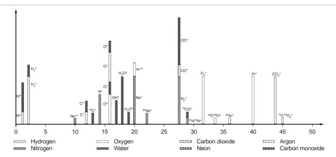
Evaluation problems: The peak at atomic number 16 may, for example, be due to oxygen fragments resulting from  $O_2$ ,  $H_2O$ ,  $CO_2$  and CO; the peak at atomic number 28 from contributions by  $N_2$  as well as by CO and CO as a fragment of  $CO_2$ ; the peak at atomic number 20 could result from singly ionized CO0 and CO1 are and double-ionized CO2.
