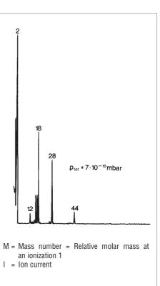
Fig. 2.57 Spectrum above a TURBOVAC 361
