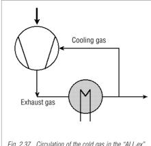
Fig. 2.37 Circulation of the cold gas in the "ALL.ex" with cooler / condenser
