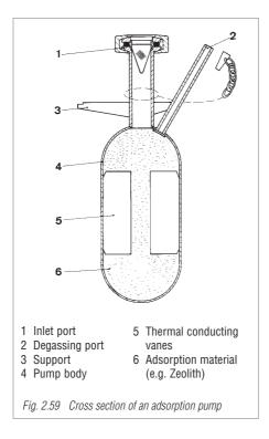
1 m². For nitrogen molecules with a relative molecular mass Mr = 28 that corresponds to about  $2 \cdot 10^{-4}$  g or 0.20 mbar · I (see also Section 1.1). Therefore, an adsorption surface of 1000 m² is capable of adsorbing a monomolecular layer in which more than 133 mbar · I of gas is bound.
