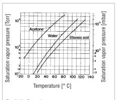
Fig. 2.15 Saturation vapor pressures
