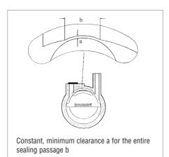
Fig. 2.4 Arrangement of the sealing passage in rotary vane pumps also known as "duo seal"
