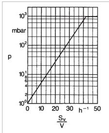
Fig. 2.58 Determination of the cut-in pressure for turbomolecular pumps when evacuating large vessels
