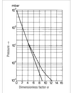
Fig. 2.75 Dependency of the dimensionless factor s for calculation of pumpdown time t according to equation 2.36. The broken line applies to single-stage pumps where the pumping speed decreases below 10 mbar
