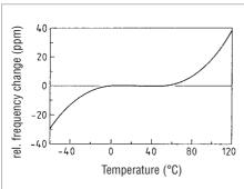
Natural frequency as a function of temperature in an AT cut quartz crystal
