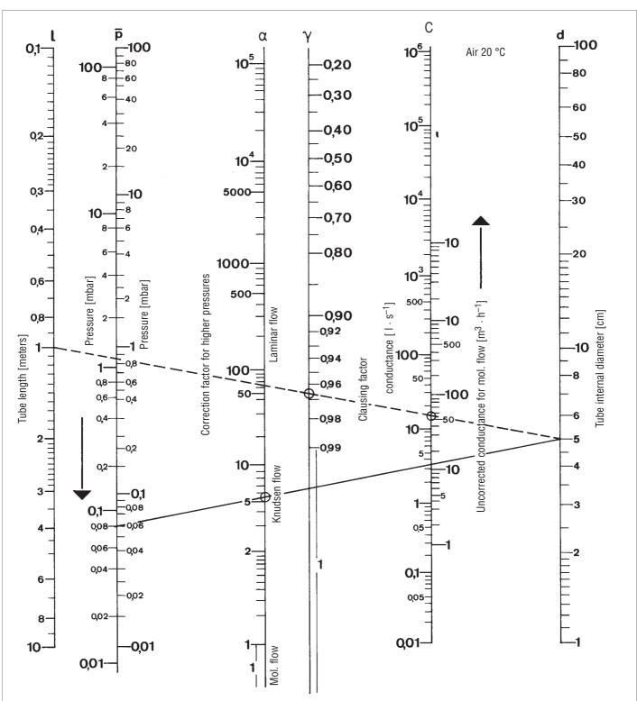
**Procedure:** For a given length (I) and internal diameter (d), the conductance  $C_m$ , which is independent of pressure, must be determined in the molecular flow region. To find the conductance  $C^{\star}$  in the laminar flow or Knudsen flow region with a given mean pressure of p in the tube, the conductance value previously calculated for Cm has to be multiplied by the correction factor a determined in the nomogram:  $C^{\star} = C_m \cdot \alpha$ .
