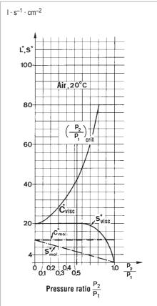
Fig. 1.3 Conductance values relative to the area,  $C^*_{ViSC}$ ,  $C^*_{moh}$  and pumping speed  $S^*_{ViSC}$  and  $S^*_{mol}$  for an orifice A, depending on the pressure relationship  $p_2/p_1$  for air at 20 °C.
