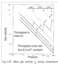
Fig. 2.32 Mean gas velocity v<sub>g</sub> during compression without purge gas (left) and with purge gas (right) in stages 2, 3 and 4
