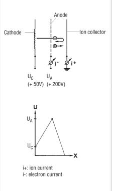
Fig. 3.13 Schematic diagram and potential curve in a hot-cathode ionization vacuum gauge
