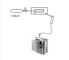
c: Integral leak detection (test gas enrichment inside the enclosure); pressurized test gas inside specimen
