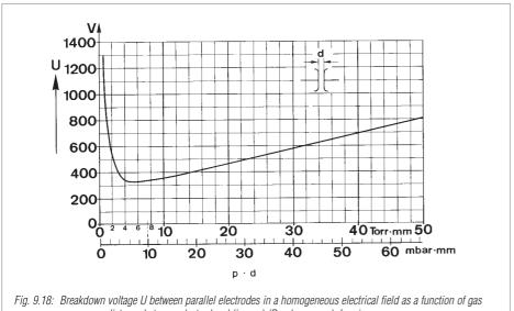
pressure p distance between electrodes d (in mm) (Paschen curve), for air
