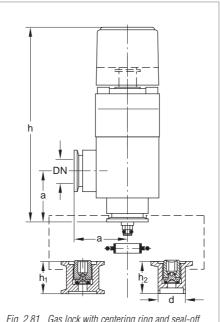
Fig. 2.81 Gas lock with centering ring and seal-off fitting sectional view
