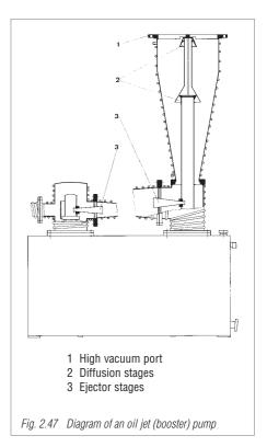
present-day vacuum technology have, in general, one or more diffusion stages and several subsequent ejector stages. The nozzle system of the booster is constructed from two diffusion stages and two ejector stages in cascade (see Fig. 2.47). The diffusion stages provide the high pumping speed between 10<sup>-4</sup> and 10<sup>-3</sup> mbar (see Fig. 2.48), the ejector stages, the high gas throughput at high pressures (see Fig. 2.49) and the high critical backing
