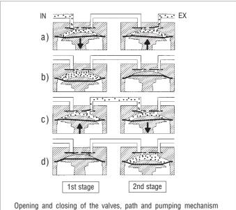
Opening and closing of the valves, path and pumping mechanism during four subsequent phases of a turn of the connecting rod (a-d)
