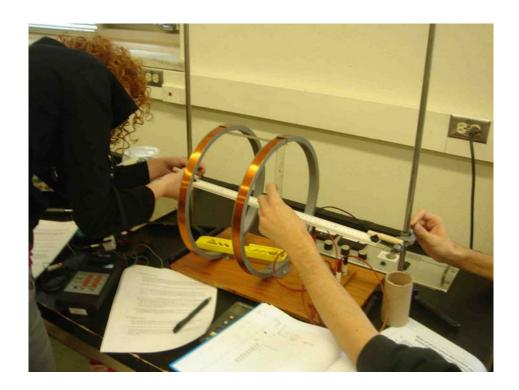
b. Position the active portion of the probe as close to the geometric centre of the coils as you can.
